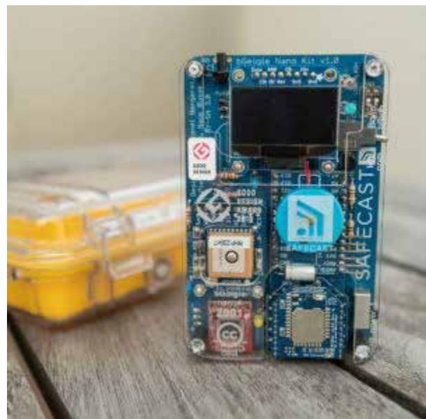
Figure 22: the bGeiger Nano, a portable handheld Geiger counter that is widely used by Safecast volunteers<sup>80</sup>
